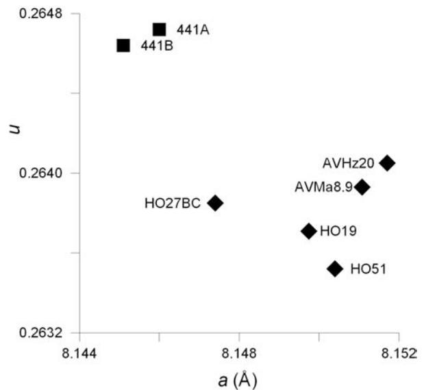
**FIGURE 4.** Oxygen fractional coordinate vs. lattice parameter.
