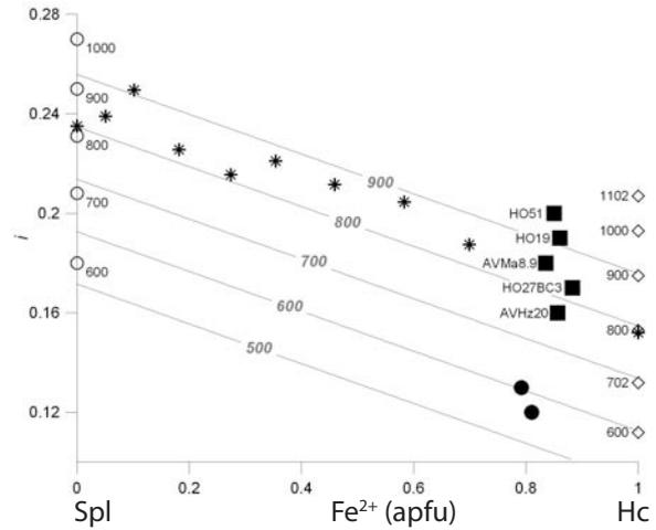
FIGURE 6. Two-dimensional projection of the  $i$ - $H_c$ - $T$  plane (fit b in Table 3) with plotted isotherms for 500, 600, 700, 800, and 900 °C. Full circles = BK samples, full squares = H&M samples. Open circles = Andreozzi et al. (2000); open diamonds = Harrison et al. (1998); asterisks = Andreozzi and Lucchesi (2002).
