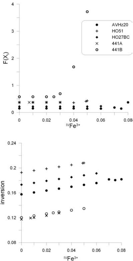
**FIGURE 2.** Plot of the minimization function (a) and of the inversion parameter (b) obtained by optimizing the distribution of Mg, Al, and  $Fe^{2+}$  with  $IVFe^{3+}$  fixed at the values in abscissa. The minimization function does not change significantly over a wide range of  $IVFe^{3+}$ , the only exception is 441B hercynite, which seems to preclude complete tetrahedral  $Fe^{3+}$  ordering.
